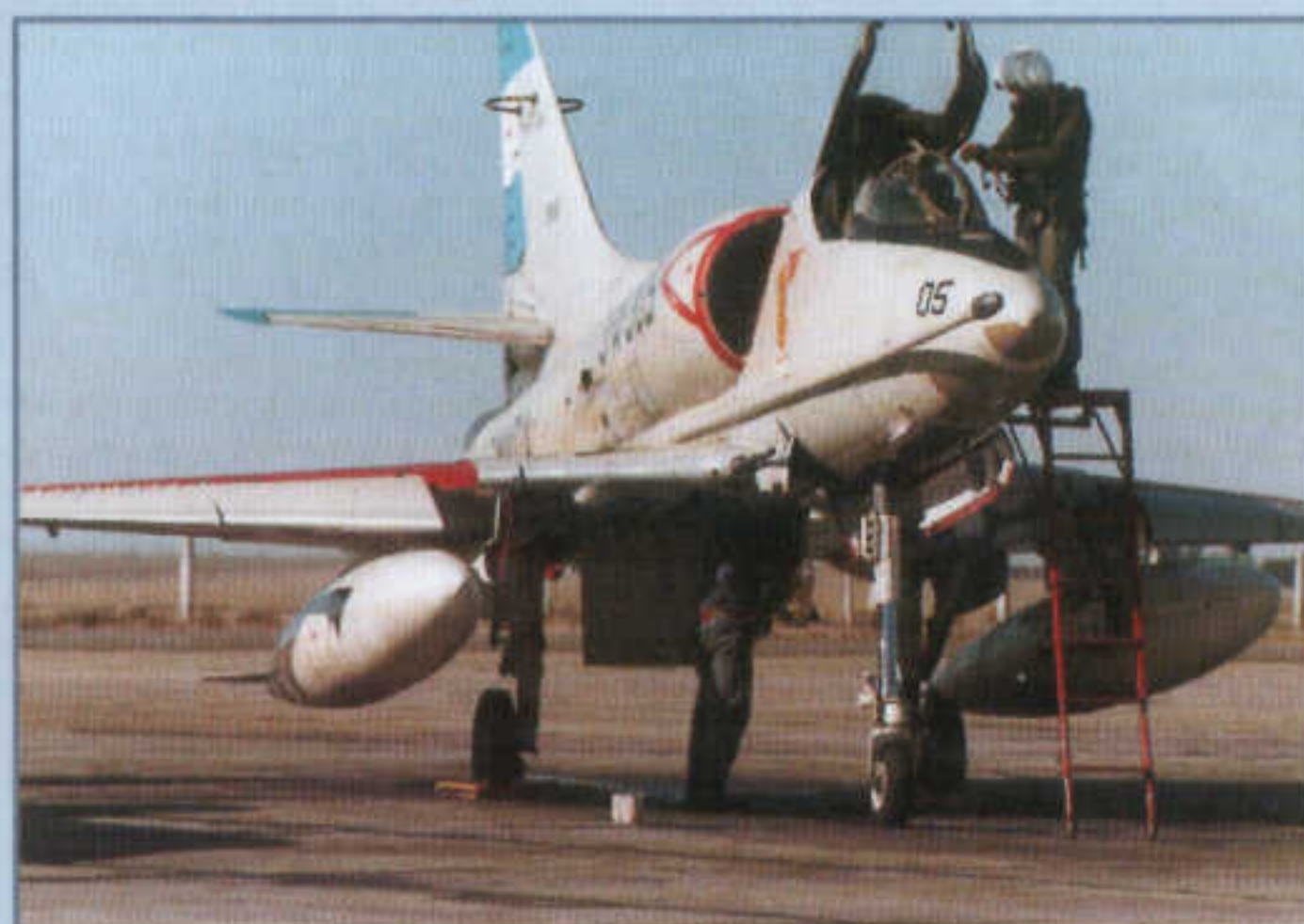
Below: A survivor of the war, A-4Q, 3-A-305, probably photographed at Rio Grande immediately after hostilities had ceased. Note how the leading edge slats droop when the aircraft is stationary. (via Jorge Felix Nunez Padin)
